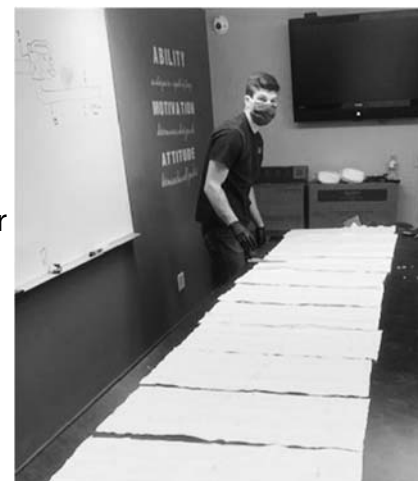
Here is 'T3' with the filter material laid out from a single Aprilaire MERV-13 filter to be cut into mask inserts that we are giving away. Filter surface area - over 28 sq.ft as shown - is the key to good air-flow in high efficiency filters. (See article below.)
