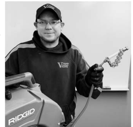
Here is Rob with our sewer cleaning system that works with our sewer video camera to pinpoint problem areas and destroy roots with the carbide-tipped chain-cutter (pictured).
