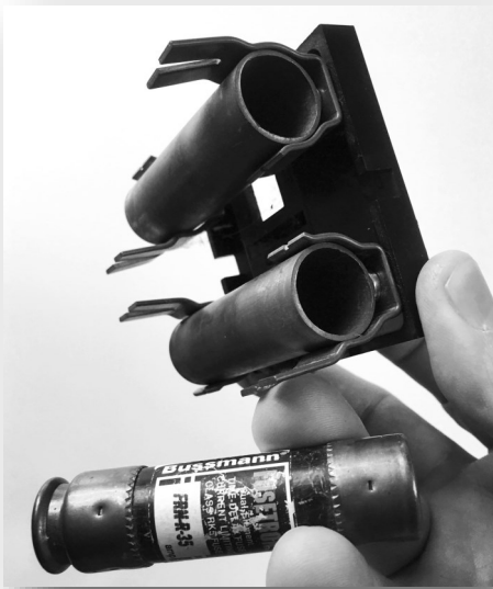
'Sabotaged' air conditioner 'disconnect' described in article with an actual cartridge fuse shown.
